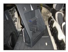
**STEP 12**Secure the driver's side plastic panel back onto the rear wall.
